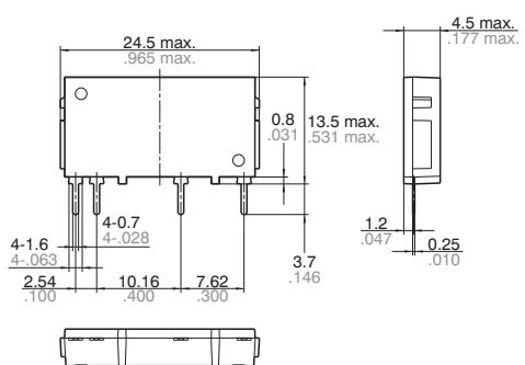
General tolerance:  $\pm 0.2 \pm .008$ **PC board pattern (Bottom view)**
