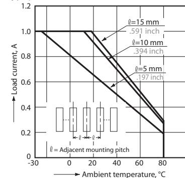
**4-(2) Load current vs. ambient temperature characteristics for adjacent mounting (2A type)**
