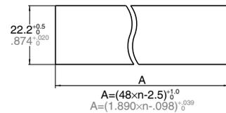
Notes: 1. Suitable installation panel thickness is 1 to 4.5 mm 0.39 to 0.177 inch.
