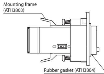
When installing the mounting frame and rubber gasket please remove the pre-attached o-ring.
