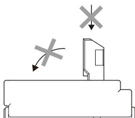
9) To close the lever, turn down the lever by pressing the entire lever or both sides of the lever with fingers tips. And close the lever completely. Be careful not to apply partial load to the lever that may cause its deformation or destruction or lever going back to initial position. Close the lever completely to prevent contact failure.
