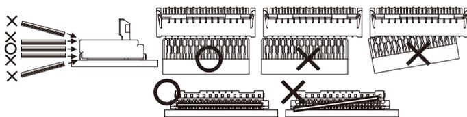
6) Insert the FPC/FFC into the connector after checking the position of FPC/FFC insertion slot and FPC/FFC. Do not insert the FPC/FFC without positioning the FPC/FFC and connector. Otherwise, it may cause connector breakages. When it is hard to insert the FPC/FFC, do not insert the FPC/FFC on that condition. Confirm the FPC/FFC and connector positioning.
