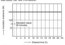
Hydrogen sulfide exposure test Test conditions: Concentration: 3 ppm Temperature: 40°C 104°F Humidity: 75% RH
